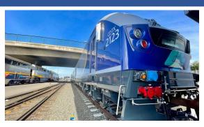
Steps in making the Capitol Corridor a greener service are underway with the pending decommissioning of two older F-59 locomotives and replacing them with Tier 4 Charger locomotives—an effort that moves us closer to a goal of 100% percent zero-emissions by 2035. *Read more*:
