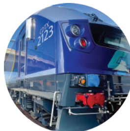
NEW CHARGER LOCOMOTIVES Two new, Tier IV Charger locomotives were added to the Capitol Corridor fleet, replacing a pair of older EPA Tier II F-59 locomotives. This brings our fleet to a total of 10 Tier IV locomotives.
